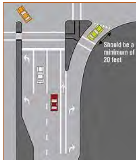
Turn Lane Striping
